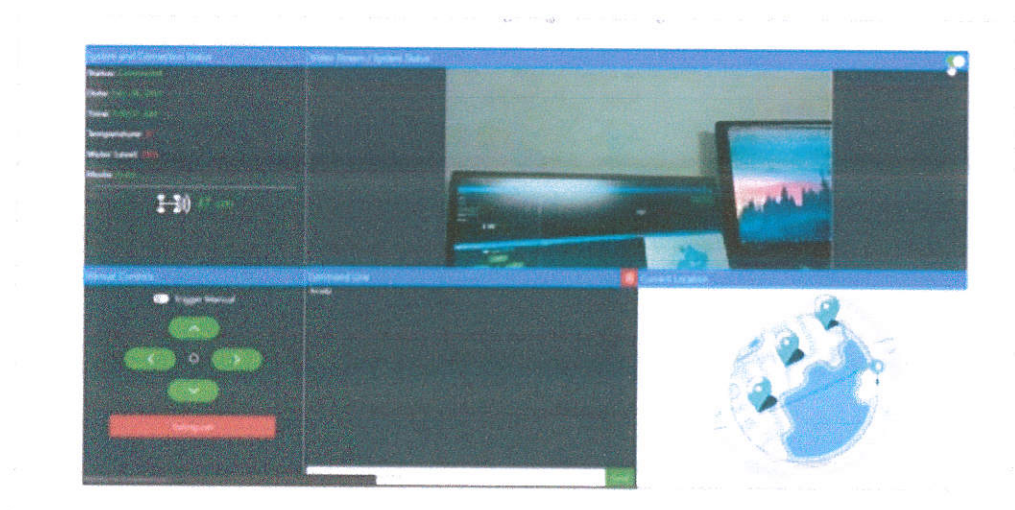
The realtime control panel and web interface for the robot
